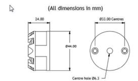
The ZTT-16-17 is mounted using two holes, on standard 33 mm fixing centres and will fit a DIN standard termination head. The ZTT-16-17 must be installed with adequate protection from moisture and corrosive atmospheres. Refer to conditions for use section of this user guide for information on enclosure IP rating.
