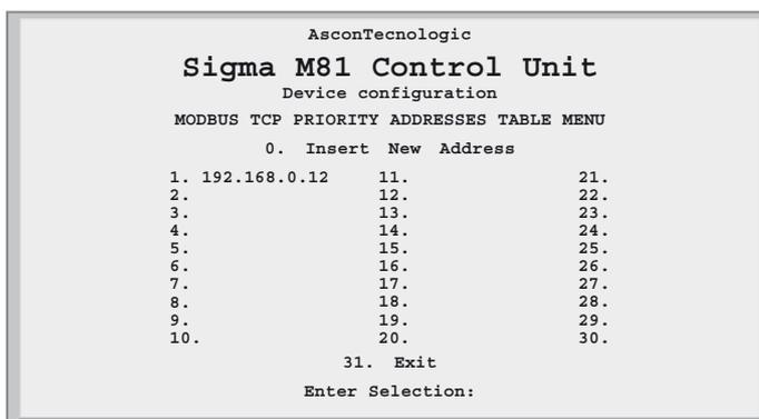
Figure 5.13 - Modbus TCP/IP Secure Addresses Table Menu
