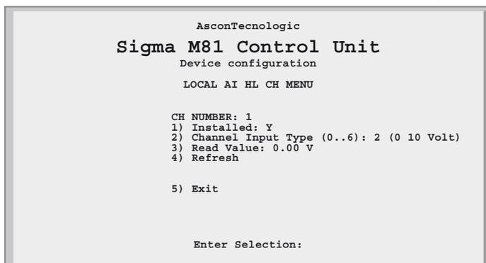
Figure 5.16 - Local Analogue Input High Level Setup Menu
