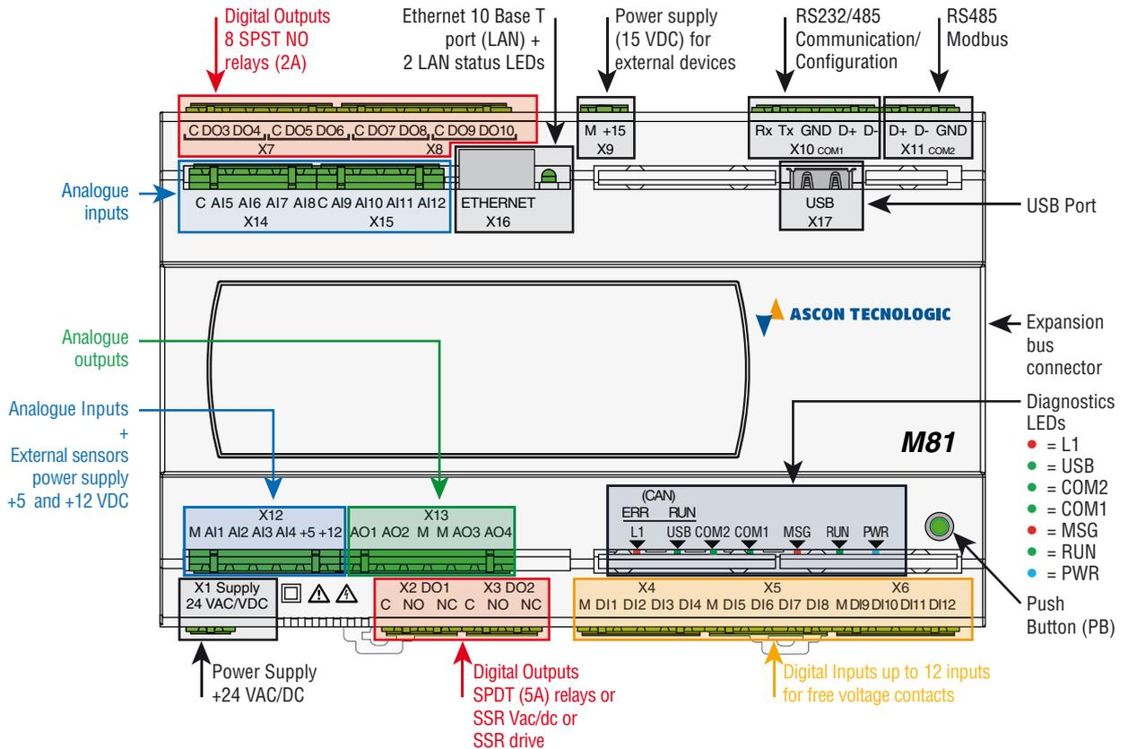
Figure 2.2 - Control Unit Supply, I/O and Communication Ports
