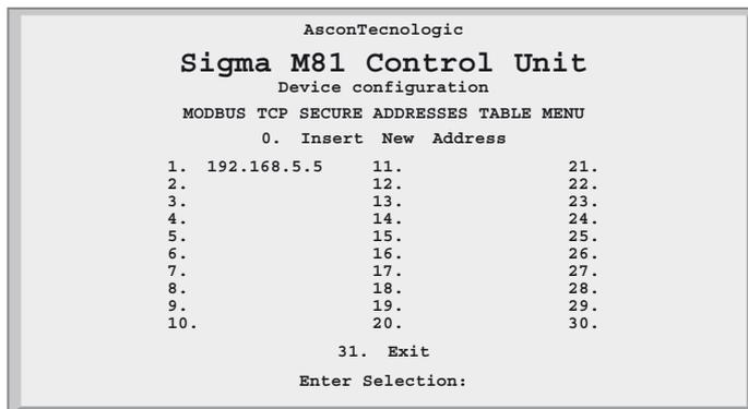
Figure 5.12 - Modbus TCP/IP Secure Addresses Table Menu
