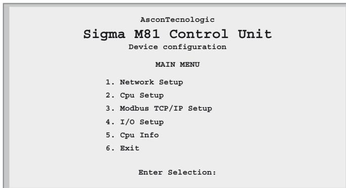
Figure 5.1 - Base Unit configuration Main Menu
