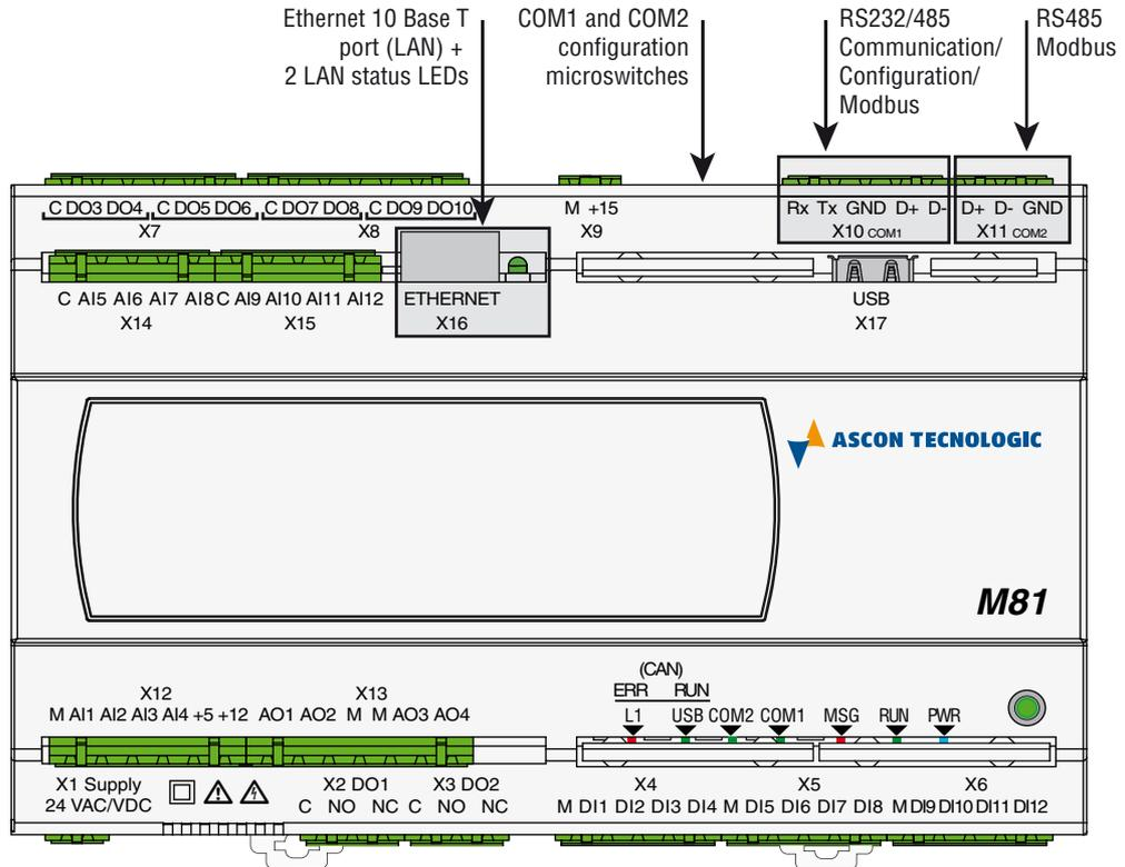
Figure 8.5 - Communication Ports and associated Protocols.
