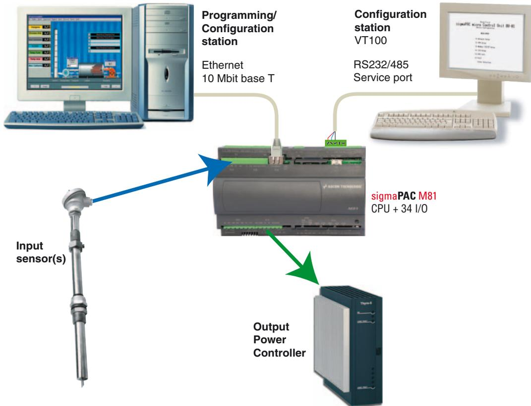
Figure 2.1 - Programming the **sigmadue M81** Control Unit
