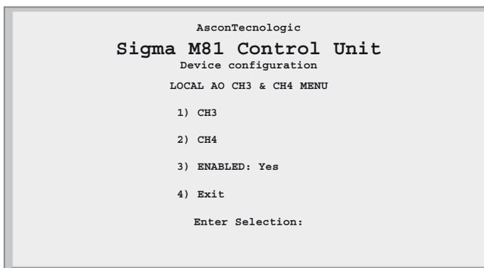
Figure 5.21 - AO Channel 3 &amp; Channel 4 Menu
