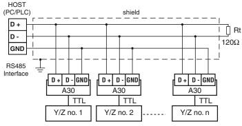
As illustrated, the line shield must be connected to ground at only one side.
