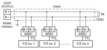
However, in particular when the network is very long or noisy and in the presence of potential differences between the various GND terminals, it is advisable to use a braided and shielded 3-pole cable connected as shown in the figure.
