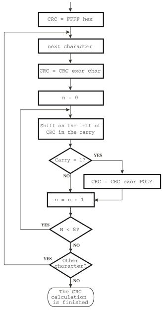
The polinomial adopted by MODBUS RTU (JBUS) is 1010 0000 0000 0001. **Note:** The first transmitted character of the CRC word is the least significant between calculated bytes.
