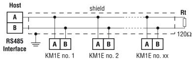
Adopted baud rates range 1200... 38400 baud, that is very satisfactory for application performances, yet very slow for RS485 interface. This fact allows the wiring of the line with a medium quality twisted pair cable: total capacity of the line should not exceed 200 nF. The line can be up to 1000 meters long.
