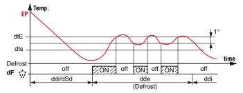
Example of electric defrost with evaporator temperature control: the defrost end after ddE programmed time. During defrost the **dF** output switch ON/OFF to control evaporator temperature in heating mode with set point dbE and 1° differential (Hysteresis).
