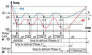
Example "dynamic defrost intervals system" with a reduction ddd = 40% and end defrost by temperature.
