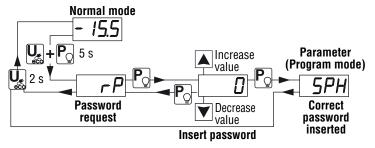
**Notes: 1.** All parameters are configured by default at "protected" level so that setting the *LPP* parameter protects all parameters with the password.
