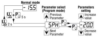
Note: With parameters in which the variable to be set is a time, the least significant time unit (s when s/min, min when min/h) is displayed in negative form (with the sign -); the most significant time unit (m when s/min, h when min/h) is displayed as a positive value (without the sign).
