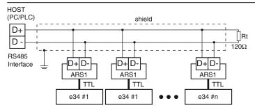
Through the **ARS1** device (TTL/RS485 interface) and the special TTL cable it is possible to connect the instrument to a RS485 serial communication network in which other instruments (controller or PLC) are inserted and typically referred to a Personal Computer used as a system supervisor.
