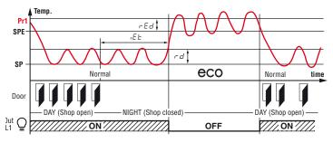
Example of automatic ECO/Normal mode activation. During the business hours the door is opened frequently and the controller remains in Normal mode. After the  ${}^{,}\mathcal{E}\mathcal{E}$  time has elapsed since the door has not been opened anymore, the controller switches to ECO mode. As soon as the door is opened again, the controller returns to Normal mode.
