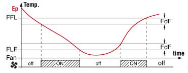
**Note:** Special attention must be paid to the correct use of the temperature-dependent fan control functions, as in a typical refrigeration application, stopping the evaporator fans blocks heat exchange.
