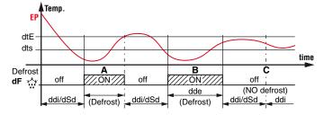
Example: Defrost **A** ends due to reaching of temperature <code>dEE</code>, defrost **B** ends at the end of the <code>ddE</code> time as the temperature <code>dEE</code> is not reached, defrosting **C** does not take place as the temperature is higher than <code>dEE</code>.
