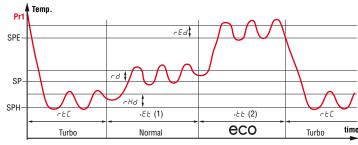
**Notes: 1.** The time 'E' is reset every time the door is opened, in the case shown the door is always closed.
