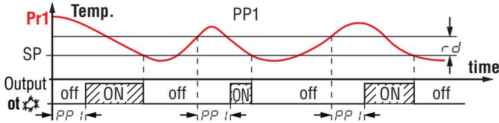
2 Second control (parameter  $PP2$ ) foresees an inhibition to the activation of the output by a time delay that starts when the output is turning OFF (delay after switching-OFF).
