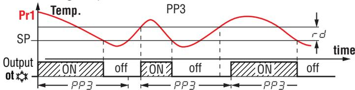
During the output inhibition the LED **OUT** (Cool ❄️ or Heat ☀️) blinks. It is also possible to prevent activation of all the outputs after the instrument is turned ON, for the time set in the parameter  $P_{od}$ .
