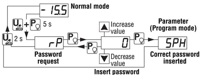
**Note:** If the Password gets lost, just switch OFF and ON the instrument, push  $\text{P/Q}$  key during the initial test keeping it pressed for 5 s. In this way it is possible to access all the parameters, verify and modify the parameter  $\text{L}^{PP}$ .
