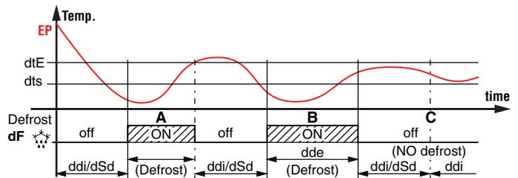
Example: Defrost **A** ends due to reaching of temperature  $dtE$ , defrost **B** ends at the end of the  $ddE$  time as the temperature  $dtE$  is not reached, defrosting **C** does not take place as the temperature is higher than  $dtS$ .
