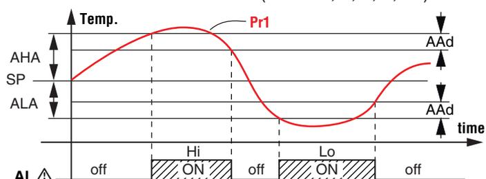
The maximum and minimum temperature alarms can be disabled by setting the related parameters *AHA* and *ALA* = **oF**.
