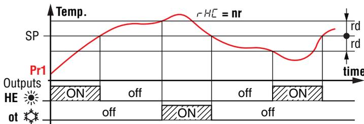
When  $r_{HC} = \text{nr}$ , the output configured as **ot** operates with a cooling action (like  $r_{HC} = \text{C}$ ) while the output configured as **HE** operates with a heating action both with the Active Set Point ( $SP_1, SP_2, SP_3, SP_4$  or  $SP_H$ ). The intervention differential ( $r_{d}/r_{Ed}/r_{Hd}$ ) is automatically
