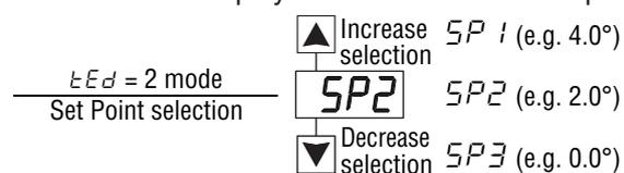
The use of the device with  $t_{Ed} = 2$  is the most practical and simple for the end user who, with the operations illustrated below, can easily select, as the active, one among the 4/5 preset Set Point temperatures ( $SPE$ ,  $SP1$ ,  $SP2$ ,  $SP3$  and  $SPH$ ).
