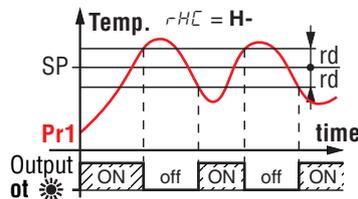
Depending on the function mode programmed with parameter  $r_{HC}$  the differential is automatically considered by the controller with positive values for a **Refrigeration** control ( $r_{HC} = \text{C}$ ) or negative values for a **Heating** control ( $r_{HC} = \text{H}$ ) or (Control with symmetrical hysteresis) with positive and negative values around the Set point for Refrigeration ( $r_{HC} = \text{C-}$ ) and Heating ( $r_{HC} = \text{H-}$ ) controls;
