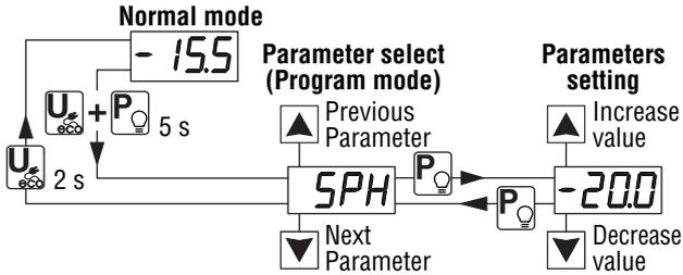
**Note:** With parameters in which the variable to be set is a time, the least significant time unit (s when s/min, min when min/h) is displayed in negative form (with the sign -); the most significant time unit (m when s/min, h when min/h) is displayed as a positive value (without the sign).
