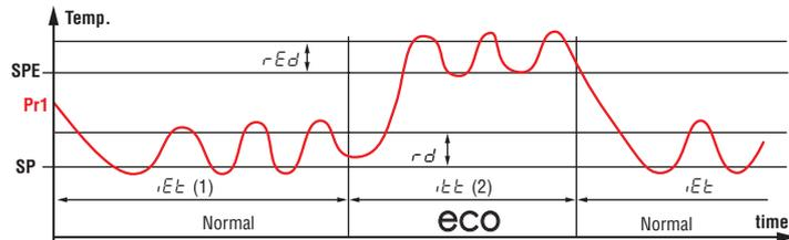
Switching to Economic mode is indicated by the label  $E_{CO}$ . In addition, the selection of the *Eco* mode is always combined with the function of turning OFF the output configured as **L1** (showcase light).
