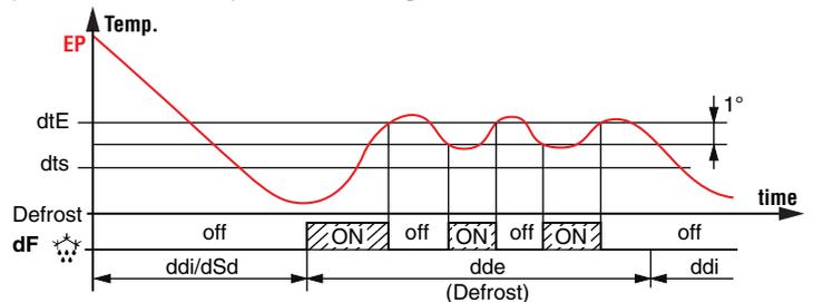
Example of electric defrost with evaporator temperature control: the defrost end after  $ddE$  programmed time. During defrost the **dF** output switch ON/OFF to control evaporator temperature in heating mode with set point  $dtE$  and  $1^\circ$  differential (Hysteresis).
