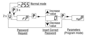
**Note:** If the Password gets lost, just switch **OFF** then **ON** the instrument, push p key during the initial test keeping it pressed for 5 s. In this way it is possible to access all the parameters, verify and modify the parameter  $\mathcal{EPP}$ .
