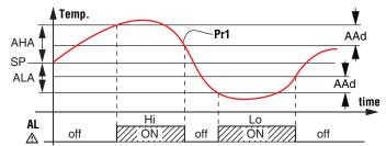
The maximum and minimum temperature alarms can be disabled by setting the related parameters RHR and RLR = oF.
