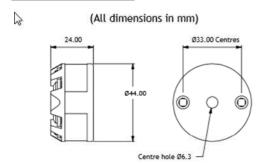
The SEM210 is mounted using two holes, on standard 33 mm fixing centres and will fit a DIN standard termination head. The SEM210 must be installed with adequate protection from moisture and corrosive atmospheres. Refer to conditions for use section of this user guide for information on enclosure IP rating.
