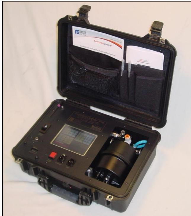
Figure 6 - Furnace Doctor® Pro Infrared gas analyzer
