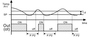
Third control (par. "**P.P3**") foresees an inhibition to the activation of the output by a time delay that starts when the output was turning on last time (delay between switching-on).
