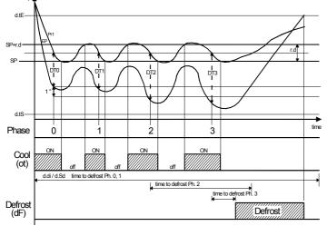
Example "dynamic defrost intervals system" with a reduction "d.dd" = 40 % and end defrost by temperature.
