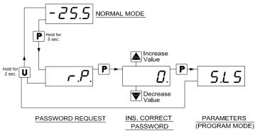
supply, push P key during the initial test and keeping the key pressed for 5 seconds.
