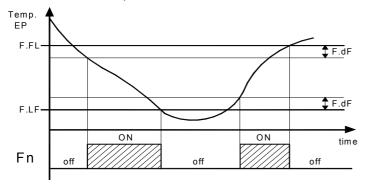
Remember that the fans functioning can be conditioned by the "Door open" function by the digital input.
