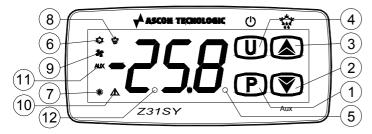
**1** - Key P : Used for setting the Set point (press and release) and for programming the function parameters (hold pressed for 5 sec.) In programming mode is used to enter in parameters edit mode and confirm the values. In programming mode it can be used together with the UP key to change the programming level of the parameters.
