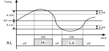
The maximum and minimum temperature alarms can be disabled by setting the relative parameters "A.HA" and "A.LA" = oF.
