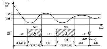
**Examples:** defrosting A ends due to reaching of temperature "dtE", defrosting B ends at the end of the "d.dE" time as the temperature "d.tE" is not reached, defrosting C does not take place as the temperature is higher than "d.tS".
