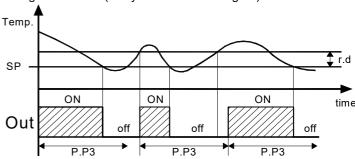
During the output inhibition the led OUT (Cool o Heat) blinking. It is also possible to prevent activation of the output after the instrument is turned on, for the time set in the parameter "**P.od**". During the power on delay phase, the display shows the indication **od.** alternating with the normal visualisation.
