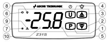
**1 - Key P**: Used for setting the Set point (press and release) and for programming the function parameters (hold pressed for 5 sec.)
