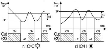
If "r.HC" = nr the output configured as "ot" work with Cooling Action (like "r.HC"=C) and the output configured as "HE" work with Heating Action
