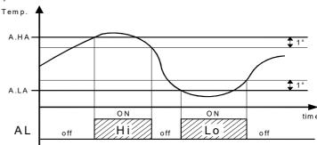
The alarm functions of the instrument work on the ALARM led, on or will be the values ["SP"+"A.HA"] and ["SP"+"A.LA"] if the alarms internal buzzer (if present and programmed by par "o bu") and on are relative ("A.Ay"=2, 4).
