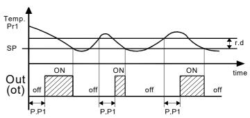
Second control (par. "P.P2") foresees an inhibition to the activation of the output by a time delay that starts when the output is turning off (delay after switching-off).
