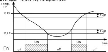
Notes: It is necessary to pay attention to the correct use of this fans temperature control functions because in the typical application of refrigeration the stop of the fans evaporator stops thermal exchange.
