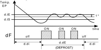
The defrost end after "d.dE" programmed time. During defrost the "dF" output switch on/off to control evaporator temperature in heating mode with set point "d.tE" and 1 ° differential (Hysteresis). The active defrost is shown on the instrument display with the
