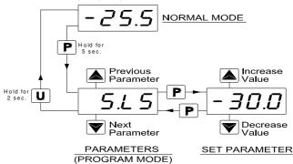
Using the UP and DOWN keys, the desired group of parameters can be selected and pressing the P key, the display will show the first parameter code of the group.
