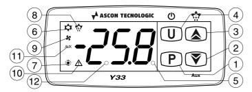
$\bf 1$  - Key  $\bf P$ : Used for setting the Set point (press and release) and for programming the function parameters (hold pressed for 5 sec.) In programming mode is used to enter in parameters edit mode and confirm the values. In programming mode it can be used together with the UP key to change the programming level of the parameters.
