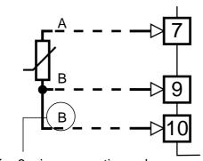
for 3-wire connection only Line: 20  $\Omega$  max. for wire
