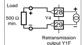
Retransmission: of measurement X of Set point W of output Y1F (Cool) Galvanically isolated 4..20mA, 10Vdc max. or
