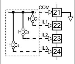
An impulsive (2 sec. at least) closing of contacts C1, C2, C3, permits the selection AUTO or MAN, Local or Remote Set point and recalling the 4 memorized Set points
