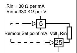
In current 4..20 mA In voltage 0..10Vdc
