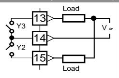
NA contacts, capacity 5A/250Vac for resistive loads (transitions 2x10 (coeff.5) min. at 5A/250Vac)
