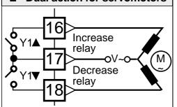
Three positions two interlocked NO (Increase stop contacts Decrease) 5A/250 Vac for resistive loads (transition 2 x 10<sup>5</sup> min. at 5A/250 Vac)
