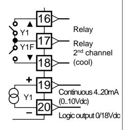
Universal and galvanically isolated. 2 relays are simultaneously present for discontinuous output with single or dual action (HEAT:COOL), or for the floating output with 3 positions for servomotors and the signal for standard continuous output 4..20mA (or 0..10Vdc) which can also be Logic output 0/18Vdc).
