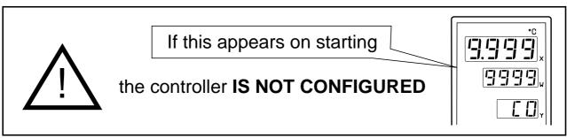
In order to configure the controller, follow the configuration procedure reported in the enclosed leaflet
