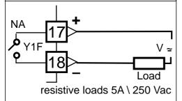
For controllers with dual action output Y1 (example: Heat-Cool), an extra output Y1F with Relay is available for the cooling action. If a continuous output is desired for cooling, use retransmission output Y4 configured for retransmission of the signal: Y1F (cool).
