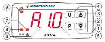
**1 - Key P**: Used for programming the function parameters (hold pressed for 5 sec.)
