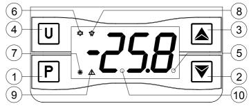
1 - Key P : Used for setting the Set point (press and release) and for programming the function parameters (hold pressed for 5 sec.) In programming mode is used to enter in parameters edit mode and confirm the values.
