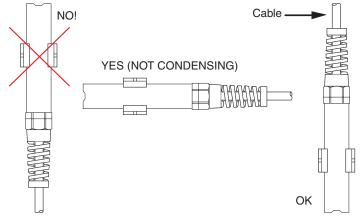
Any error in humidity measurement may be due to the settling time of the probe, in this case it will be necessary to wait for the time necessary to achieve a stable measurement. Steam jets, water sprays, drafts, direct sun exposure, condensation on the sensor or mounting on a wall made cold by the outside temperature can also cause important measurement errors; due to these conditions, during the installation, the probe must be protected from any possible external influence.
