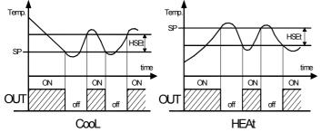
In the event of probe error, it is possible to set the instrument so that that the output "OUT" continues to work in cycles according to the times programmed in the parameter "tonE" (activation time) and "toFE" (deactivation time).
