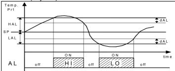
The maximum and minimum temperature alarms can be disabled by setting the relative parameters "HAL" and "LAL" = OFF.
