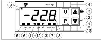
${\bf 1}$  -  ${\bf Key}~{\bf P}$  : Used for setting the Set point and for programming the function parameters
