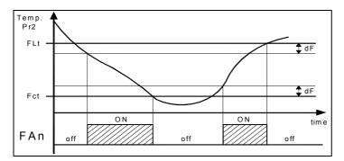
When the probe Pr2 is used (par. "Pr 2" = on) the fans, as well as being conditioned by the parameters "FCOF" and "FEdF", are also conditioned by the temperature control.
