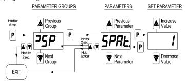
The instrument has a parameter protection function using a password that can be personalised, through the "PASS" parameter in the "**PAn**" set.
