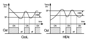
In the event of cell probe error (Pr1), it is possible to set the instrument so that that the output "Out" continues to work in cycles according to the times programmed in the parameter **"tonE"** (activation time) and **"toFE"** (deactivation time).
