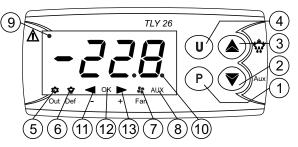
1 - Key P: Used for setting the Set point and for programming the function parameters
