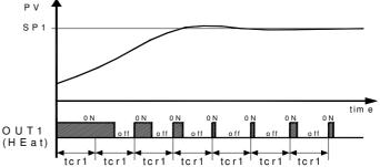
In order to obtain good stability of the process variable, in the eve of fast processes, the cycle time "tcr1" has to have a low value wi a very frequent intervention of the control output.
