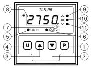
**1 - Key P** : Used to access function programming parameters and to confirm selection.
