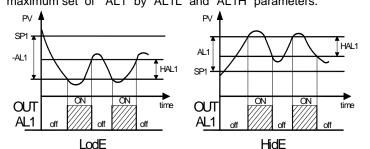
LHAb = ABSOLUTE BAND ALARM: The alarm is activated when the process value goes under the alarm threshold set on parameter "AL1L" or goes higher than the alarm threshold set on parameter "AL1H" and will be deactivated when it goes below the value [AL1H - HAL1] or when it goes above the value [AL1L + HAL1].
