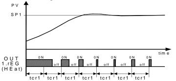
In order to obtain good stability of the process variable, in the event of fast processes, the cycle time "tcr1" has to have a low value with a very frequent intervention of the control output.
