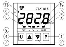
${\bf 1}$  -  ${\bf Key}~{\bf P}$  : This is used to access the programming parameters and to confirm selection.
