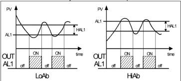
LodE = DEVIATION LOW ALARM: The alarm is activated when the ways depending on the value added to par. "Ab1". process value goes below the value [SP + AL1] and will be deactivated when it goes above the value [SP + AL1 + HAL1].
