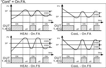
The control works in the following way : in the case of reverse action, or heating ("FunC"=HEAt), it deactivates the output, when the process value reaches [SP + HSEt] in case of symmetrical hysteresis, or [SP] in case of asymmetrical hysteresis and is then activated again when the process value goes below value [SP -
