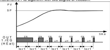
of fast processes, the cycle time "tcr1" has to have a low value with a very frequent intervention of the control output.
