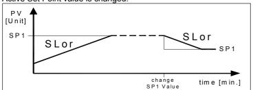
If it is desired an automatic cycle from the power on instead it is necessary to program the par. "nSP" = 2, to program the two Set Point values "SP1" and "SP2" and naturally to program the par. "SLor", "dur.t" and "SLoF" with the desired values.
