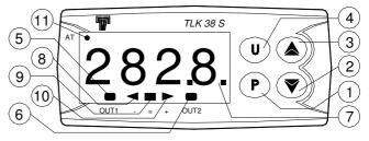
1 - Key P : This is used to access the programming parameters and to confirm selection.
