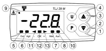
${\bf 1}$  -  ${\bf Key}~{\bf P}$  : Used for setting the Set point and for programming the function parameters
