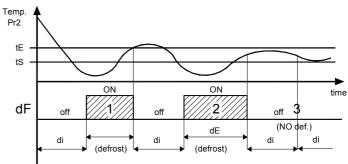
**Examples:** defrosting 1 ends due to reaching of temperature "tE", defrosting 2 ends at the end of the "dE" time as the temperature "tE" is not reached, defrosting 3 does not take place as the temperature is higher than "tS".
