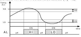
All the parameters concerning the alarm functions are contained in or will be the values ["SP"+"HA"] and ["SP"-"LA"] if the alarms are relative ("Ay"=dE).
