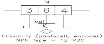
n order to the counting frequency is advisable to program the filter software of the par. "H" that it allows to select the maximum counting requency and to avoid
