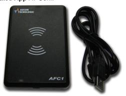
To configure the instrument with the **NFC**, it is not necessary to power the timer, but simply put its front panel on the symbol ((\*)) of the **AFC1** device surface (which is powered directly by the **USB** port connected to the **PC**) or on the smartphone part on the which is the **NFC** interface (for this consult the smartphone user manual) then send the parameters to the instrument memory.
