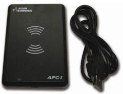
To configure the instrument with the **NFC**, it is not necessary to power the timer, but simply put its front panel on the symbol ((\* )) of the **AFC1** device surface (which is powered directly by the **USB** port connected to the **PC**) or on the smartphone part on the which is the **NFC** interface (for this consult the smartphone user manual) then send the parameters to the instrument's memory.
