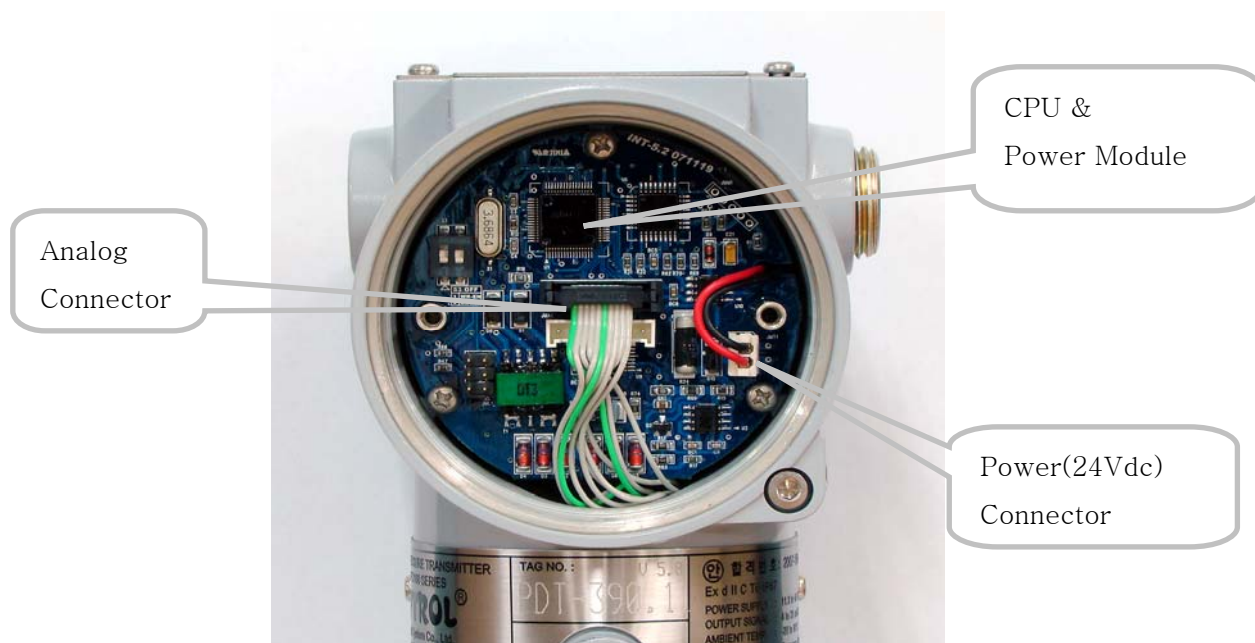
Figure 6.3 Structure of Electronics Module inner Transmitter
