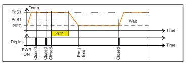
When a new panel is detected before the end of the first soak time, the program restarts and the set point remains equal to Pr.S1.
