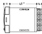
The controllers with universal power supply, have the body long 63.3 mm
