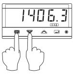
Press simultaneously for 2 seconds
