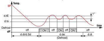
Example of electric defrost with evaporator temperature control: the defrost end after the ddE programmed time. During defrost the **dF** output switches ON/OFF to control evaporator temperature in heating mode with set point ddE and 1° differential (Hysteresis) to maintain the temperature close to ddE. At defrost end of, it is possible to delay the new compressorstart up (**ot** output) at the time set at parameter ddd to allow the evaporator to drain.
