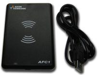
To configure the instrument with the **AFC1** device, the instrument must be placed on the side indicated with the appropriate symbol on the AFC1 device, which is powered directly by the USB port connected to the PC.
