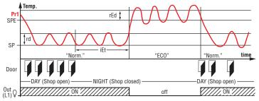
The *Normal/Economic* mode can be selected automatically or manually via the digital input when  $\sqrt{F}_{ij} = 6$ :
