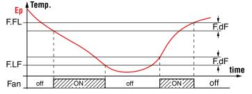
**Note:** It is necessary to pay attention to the correct use of this fans temperature control functions because in the typical application of refrigeration the stop of the evaporator fans stops also the thermal exchange.
