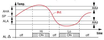
The maximum and minimum temperature alarms can be disabled by setting the related parameters RHR and  $RLR = \mathbf{oF}$ . The temperature alarms are signalled lighting up the alarm LED.
