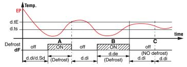
Defrost end example: Defrost **A** ends due to reaching of temperature <code>def.</code>, defrost **B** ends at the end of the <code>ddE</code> time as the temperature <code>def.</code> is not reached, defrosting **C** does not take place as the temperature is higher than <code>def.</code>.
