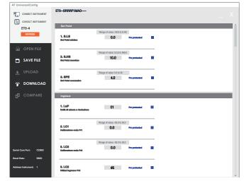
The transmission of the parameter configuration to the instrument can take place via the TTL communication port and the A01 device or, if the instrument is equipped with the optional NFC communication, by means of the AFC1 device. The A01 and AFC1 devices are connected to the PC via a common USB port.
