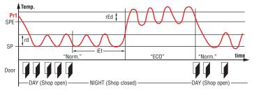
The Normal/Economic mode can be selected automatically or manually via the digital input when  $\sqrt{r} = 6$ :
