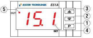
P: Used for setting the Set point (short press) and for programming the function parameters (pressed for 5 s). In programming mode is used to enter in parameters edit mode and confirm the values. In programming mode can be used together with the key to change the programming level of the parameters. When the keyboard is locked, the keys and sused together (hold pressed for 5 s), unlock the keyboard.
