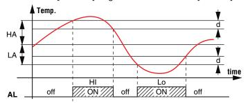
In alarm condition the instrument shows on the display:  $\mathcal{H}$ , alternated to the measured temperature(max. alarm);  $\mathcal{L}_{\mathcal{D}}$  alternated to the measured temperature (min. alarm). The maximum and minimum temperature alarms can be disabled by setting the related parameters  $\mathcal{H}\mathcal{B}$  and  $\mathcal{L}\mathcal{B} = \mathbf{oF}$ .
