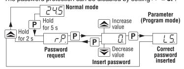
**Note:** If the Password gets lost, just just cut OFF the supply, then push  $\begin{tabular}{l} {\bf P} \end{tabular}$  key and keep it pressed for 5 s while powering again ON the instrument. In this way it is possible to access all the parameters, verify and modify the parameter  $\begin{tabular}{l} {\cal PP}. \end{tabular}$
