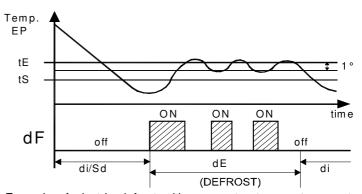
Example of electric defrost with evaporator temperature control: The defrost end after "dE" programmed time. During defrost the "dF" output switch on/off to control evaporator temperature in heating mode with set point "tE" and 1 ° differential (Hysteresis).
