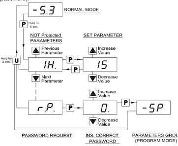
In case some parameters are not protected, when one tries to have access at the programming, the display will show all the parameters not protected and the par. "r.P" (through which will be
