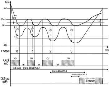
Example "dynamic defrost intervals system" with a reduction "dd" = 40 % and end defrost by temperature.
