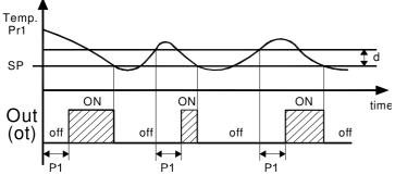
Second control (par. "P2") foresees an inhibition to the activation of the output "ot" by a time delay that starts when the output is turning off (delay after switching-off).
