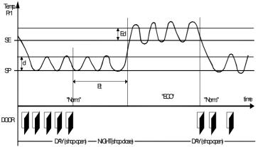
Example of automatic switching between Eco mode and normal mode. During working hours the door is frequently opened and the controller stays in normal mode. When the door has not been opened for time "Et", the controller switches to Eco mode. As soon as the door is opened again, the controller reverts to normal mode. This function requires use of a digital input configured as "xF" = 1, 2 or 3 (door open input)
