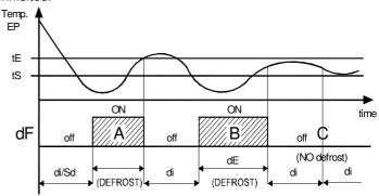
Examples: defrosting A ends due to reaching of temperature "tE", defrosting B ends at the end of the "dE" time as the temperature "tE" is not reached, defrosting C does not take place as the temperature is higher than "tS".
