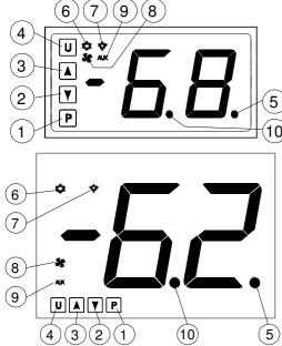
1 - Key P: Used for setting the Set point (press and release) and for programming the function parameters (hold pressed for 5 sec.) In programming mode is used to enter in parameters edit mode and confirm the values. In programming mode it can be used together with the UP key to change the programming level of the parameters.
