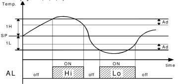
The maxima and minima temperature alarms can be disabled by setting the relevant parameters "A.Hx" and "A.Lx" = oF.
