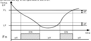
It is possible to set the disablement of the fans when the temperature measured by the evaporator probe is higher than the one set in the parameter "FL" (temperature too hot) or when it is These parameters are:
