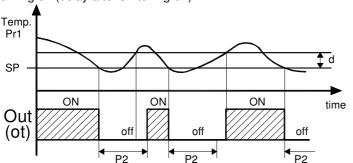
Third control (par. "P3") foresees an inhibition to the activation of the output "ot" by a time delay that starts when the output was turning on last time (delay between switching-on).
