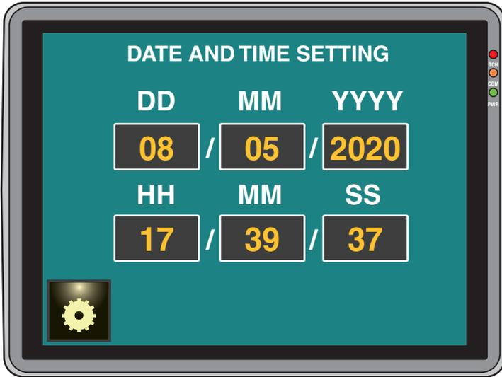
To set the current date and time tap on the desired parameter (DD = day, MM = month, YYYY = year, HH = hour, MM = minute, SS = second); the system at this point shows a numeric keypad to insert the desired value.
