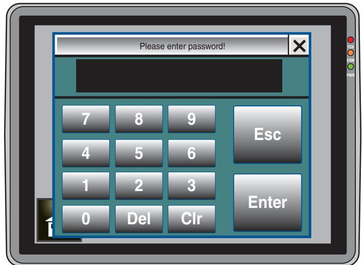
Set the correct password number and press . If the password is correct the system will enter the previously selected page.
