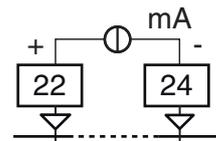
**mA output:** 0/4... 20 mA, galvanically isolated, RL max. 600Ω.
