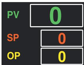
Tapping the set point window it is possible to change its value while the present value and the output power can only be read.
