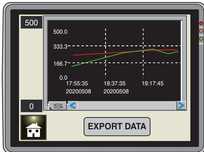
The RED line represents the Set Point trend while the GREEN one represents the temperature Measurement over the time.
