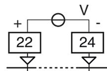
**V output:** 0/2... 10 V, galvanically isolated, RL min.: 500Ω.
