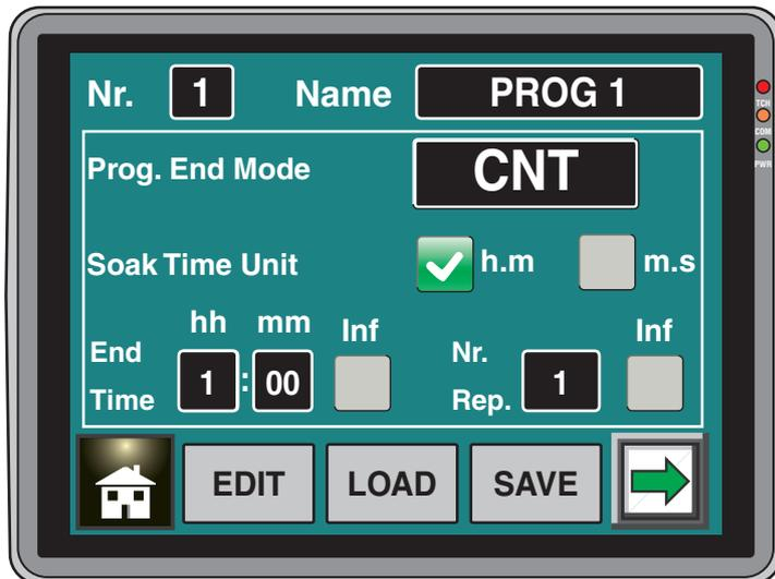
In order to modify the values assigned to the various parameters, it is necessary to tap on the **EDIT** button. At this point the system displays the following page:
