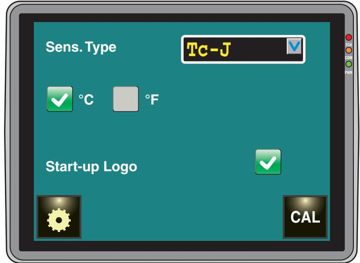
In the **Sens. Type** field, select the desired probe type.
