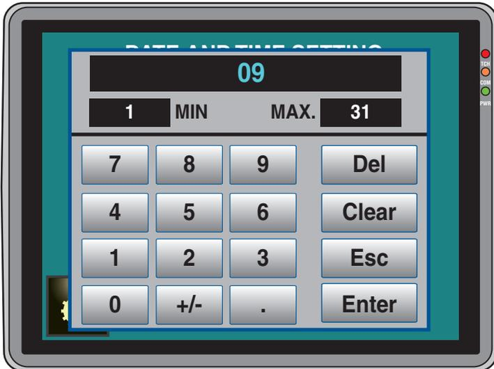
At the top is shown the present value, then the minimum and maximum allowed values. Functions of the keys on the right:
