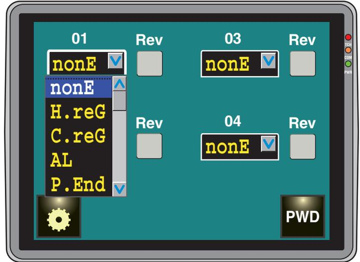
**Range: nonE** Output not used. With this setting the status of this output can be set through the serial interface;
