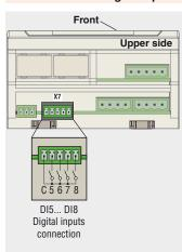
Example of connection of DI5... DI8 Digital Inputs.
