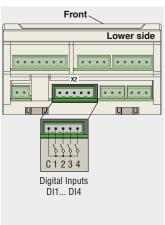
Example of connection of DI1... DI4 Digital Inputs.
