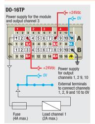
Protect loads with fast type fuses adequate to the power consumption of each load (4A max.)
