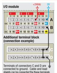
An additional terminal block can be installed on the I/O module using the two slides located in the lower part of the module case (item 11 in "General description" paragraph).
