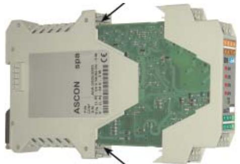
Bornier de raccordement
