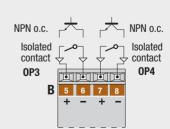
When terminals 5, 6 and 7, 8 are not configured as OP3 and OP4 outputs, they can be used as voltage or isolated contact inputs.
