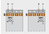
\Lambda When terminals 5, 6 and 7, 8 are not configured as OP3 and OP4 outputs, they can be used as voltage or isolated contact inputs.
