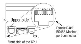
The RS485 Modbus Port can be used to connect a Modbus fieldbus. The RJ45 RS485 Modbus Port connector is located in the upper side (on the left) of the CPU (see "2-2-2 MP-02 CPU" on page 15). Looking the hole of the plug the 8 contacts are arranged as illustrated in the draw.
