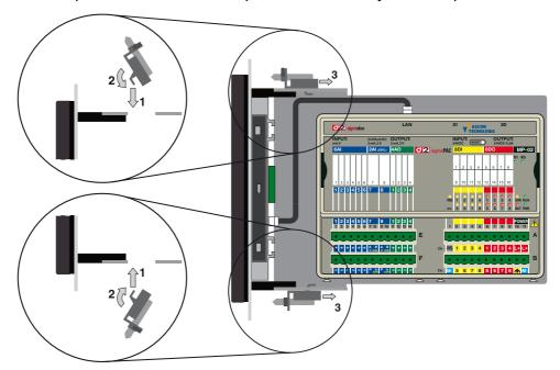
Rotate clockwise the clamps screws until the instrument is firmly locked to the cabinet panel. Do not over tighten the screws, to avoid panel distortions.
