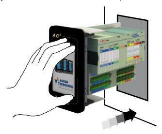
• Fit the two mounting clamps, fixing them in the slots at the top and bottom side of the the metal plate. To hook the clamps, slide them away from the panel;
