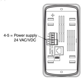
The power supply is to be provided to the operator panel via terminals 4 and 5 of the terminal block. Since the power required can be both in alternate and in direct current (AC/DC), the polarization of the terminals is irrelevant. The power supply terminals ar fully isolated from the communication connectors.
