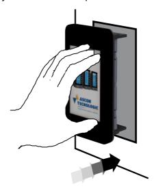
Insert the four mounting clamps, in the rear side of the P04 Operator Panel as illustrated;
