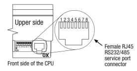
The RS232 Service Port can be used to configure the CPU and its devices using a dumb VT100 terminal. The RJ45 RS232/485 Service Port connector is located in the upper side (on the right) of the CPU (see "2-2-2 MP-02 CPU" on page 15). Looking the hole of the plug the 8 contacts are arranged as illustrated in the draw.
