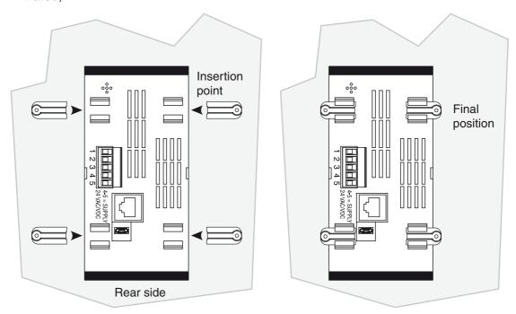
Now mount a retaining screw in the hole present in each clamp;
