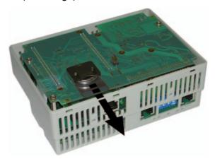
Replace the battery with the positive pole facing the rear panel of the CPU and the negative one in contact with the printed circuit (see image).
