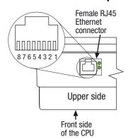
The Ethernet TCP/IP port RJ45 connector is located in the upper side of the CPU (see "2-2-2 MP-02 CPU" on page 15). Looking the hole of the plug the 8 contacts are arranged as illustrated in the draw.
