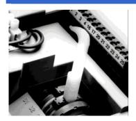
For cam adjustment the proper lever supplied with the gear motor equipment is to be used. Use the lever from the right side, introducing the pin into one of the bores on the sides of the blue cam and lever it to the desired position.
