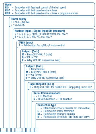
\*: For servomotor drive, both OUT 1 and OUT 2 codes must be selected as "M".
