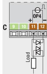
Double action Relay (SSR) / Relay (SSR)
