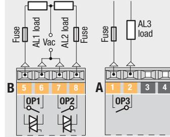
**The relay/SSR output OP1, OP2 and OP3, can be used as alarm outputs only if they are not used as control outputs**
