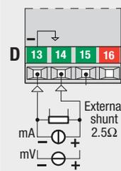
PV control input with 2 wires transducers
